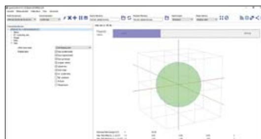
LPMS is visualized as a 3D sphere. A bar graph indicates the current magnetic noise level in real-time.
